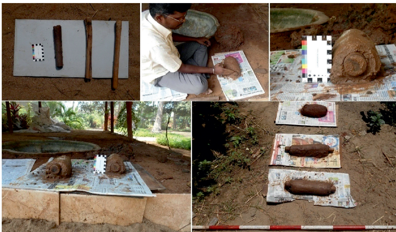
Fig. 7: Preparation of Tuyeres
